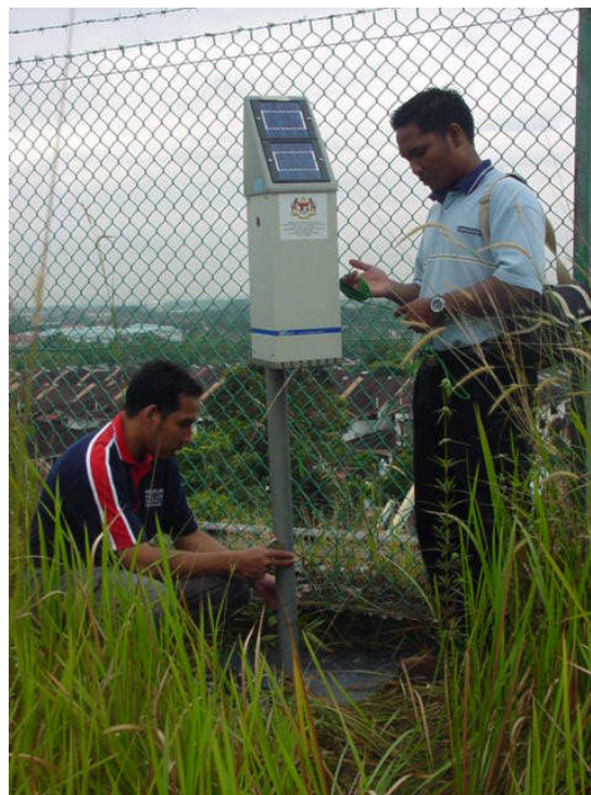
Figure 2. Set-up of PMM instrument Model 8055 with probe model PMM EP-33M for 24 hours monitoring.
