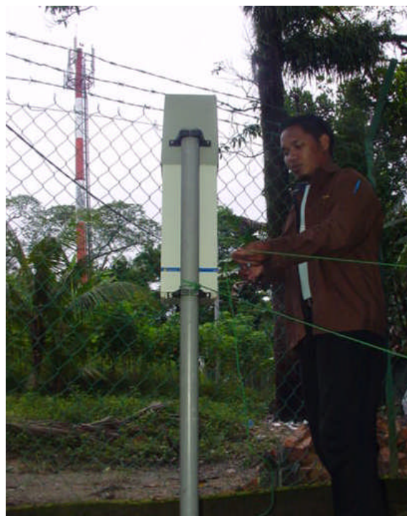
Figure 2. PMM instrument Model 8055 with probe model PMM EP-33M (for 24 hours monitoring)
